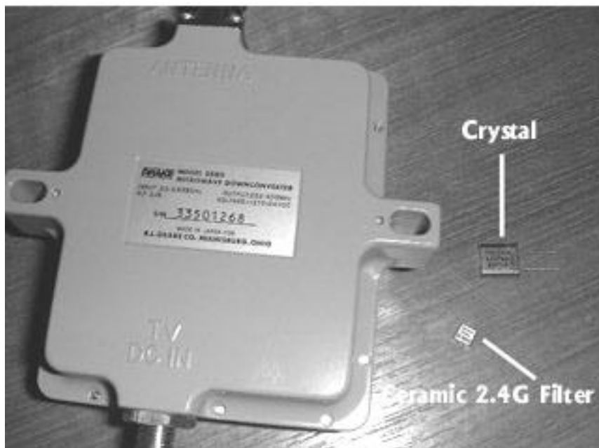
Figure 1. Drake 2880 converter together with replacement crystal for the PLL and the ceramic 2.4GHz RF filter
