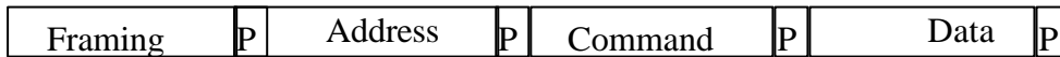
Fig 2 The basic messages format consisting of 3 bytes plus an additional data byte with a single odd parity bit between each byte.
