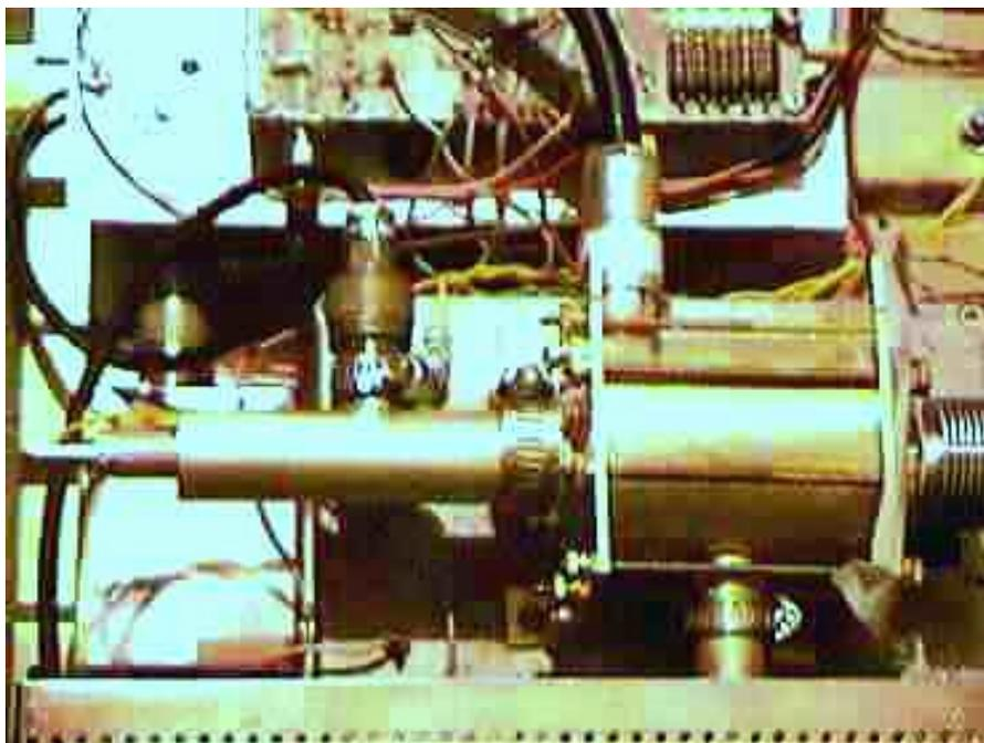
PCS Power Amplifier – before modification, PA Transistor above left end of blue power module
