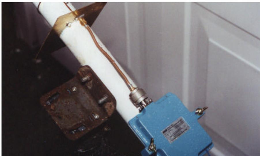
The claimed calculated gain figure for this aerial is about  $10 \times \log ( 15 \times 20 \text{ (turns)} \times \tan(12.5)) = 18.2\text{dBi}$ . It is generally accepted that these calculated gain figures are in the order of 1 to 2dB too high. (However read Kent Britains article above – no guarantees implied!)
