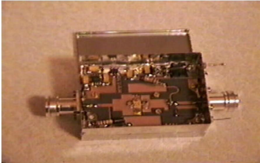
K9EK Amplifier in G3XDY 2.3GHz Transverter
