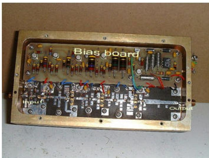
After trying unsuccessfully to replace the blown input FET I tried the more practical approach of merely strapping out the input stage. First, check this is where the fault is. (You can be better than 90% certain it will be). It is easy to prove this is the stage at fault as the bias condition around the device will be found to be inconsistent with, usually, the negative gate bias voltage on the first stage non-existent.
