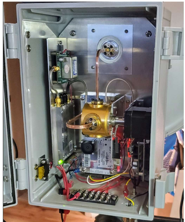
Motorised waveguide switch Hugh VA3TO
