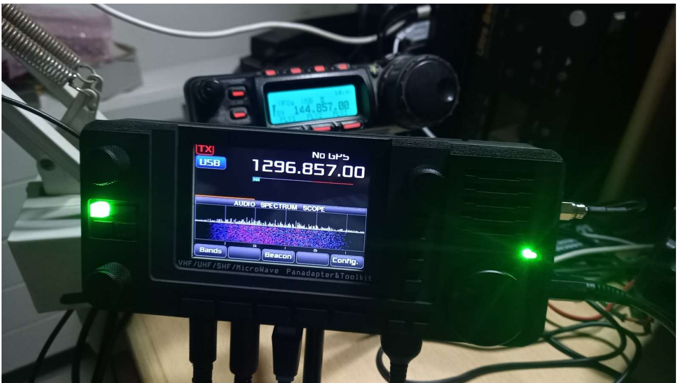
Maxicom connected to an FT857 using a 23cm transverter
