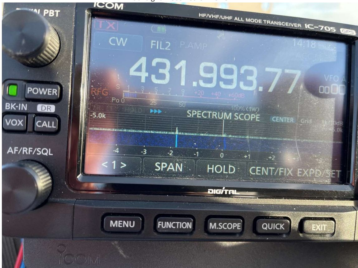
122GHz 2mW signal from Noel on the left. Just to the right of centre, is the signal from Neil G4LDR's 'VK' system.
