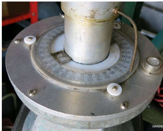
Figure 1 Rotatable protractor on dish tripod (the protractor rollers and bed are made of PTFE)
