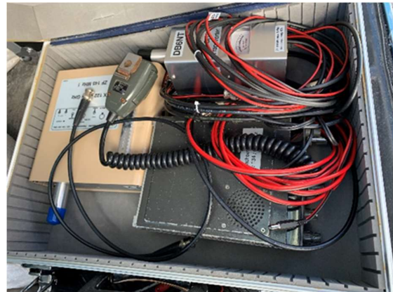
2x battery, case for FT-290 und 76 GHz Transverter and big case for mmWave-station with dish
