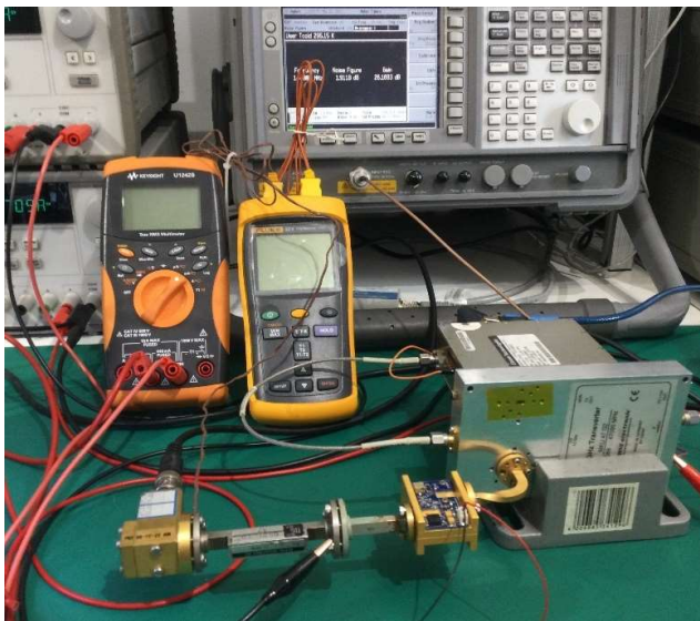
47GHz LNA Number 1, showing 1.9dB NF and 26dB gain.
