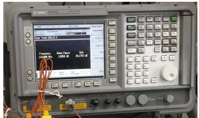
47GHz LNA Number 1, showing 1.9dB NF and 26dB gain.
