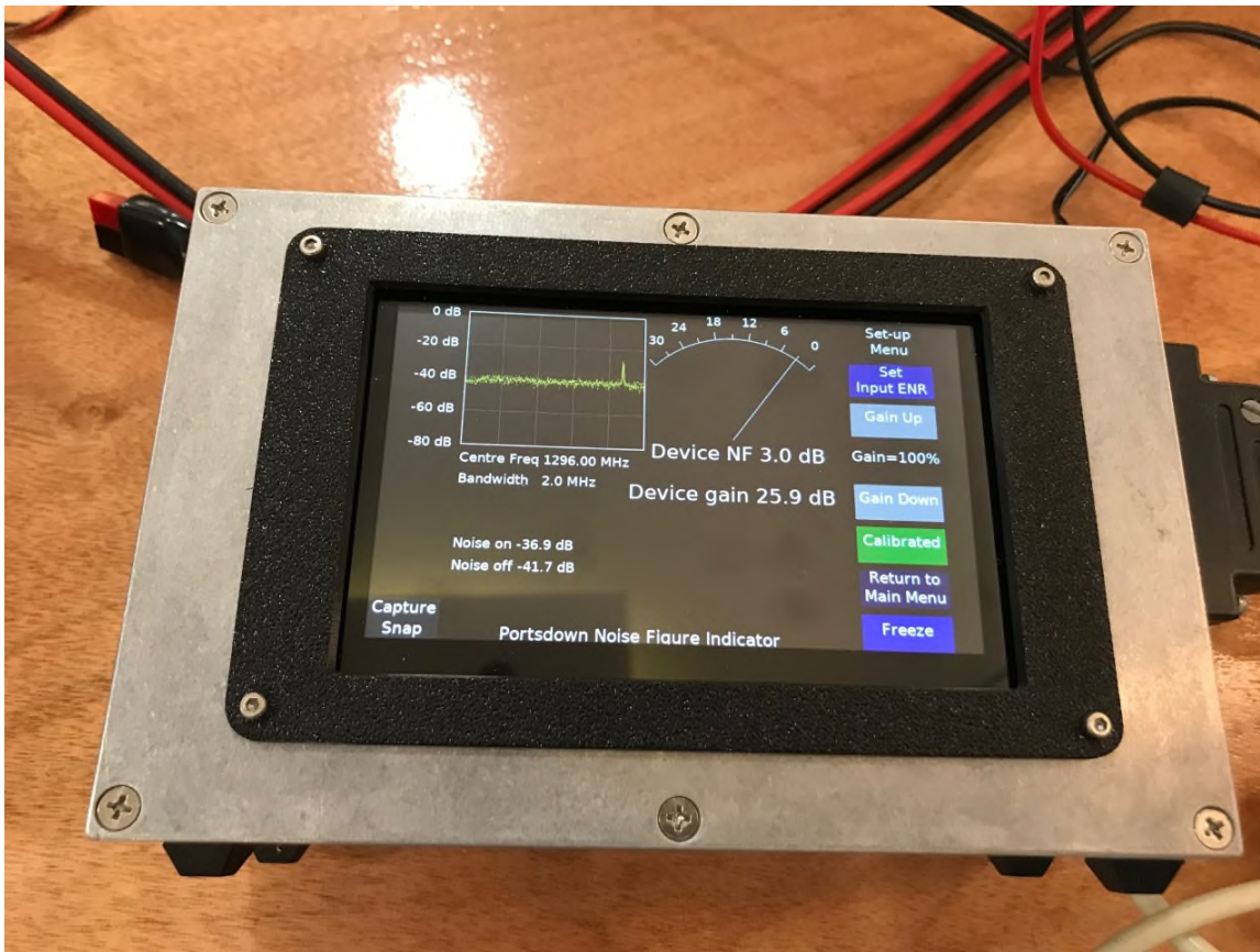
An example of a Portdown working as a Noise Figure meter. As described by Dave G8GKQ in his test equipment talk.
