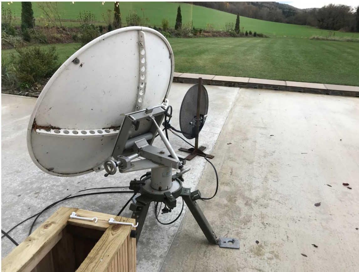
QO100 beautifully engineered dish belonging to John G7ACD in use throughout.
