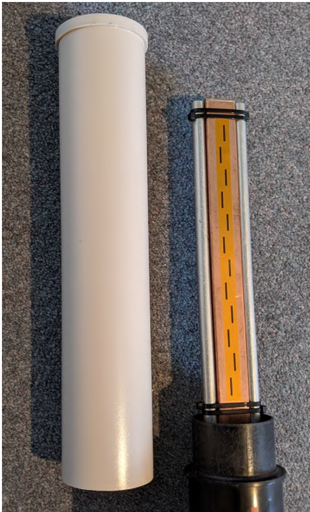
Antenna with protective radome
