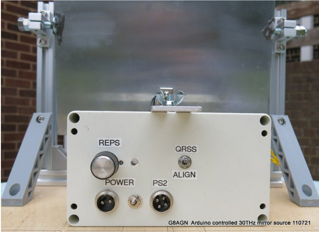
Photo 3 – Front panel of control box. The REPS knob controls the number of times that a message is sent
