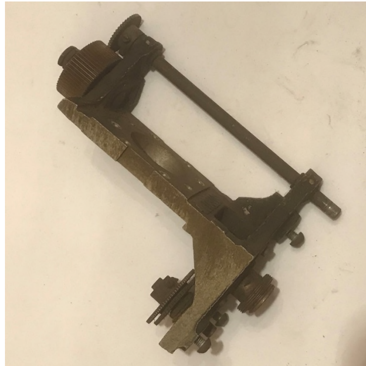
Fig 8 The substantial cast aluminium mounting frame, which also served to heat sink the klystron
