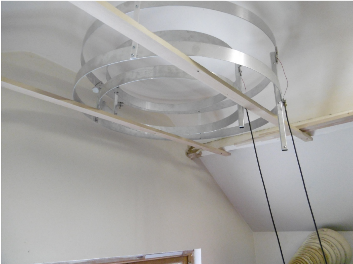
Figure (3) Nested 50 and 70MHz vertically polarized slot antennas in a loft 1dBd omni. Much more convenient than a half wave dipole. Copyright G3WRT
