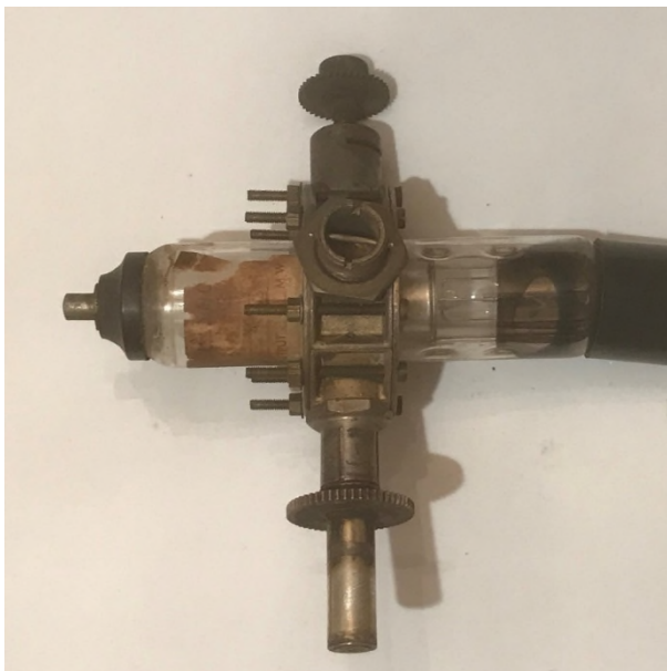
Fig 7. Removed from the frame work: at the top is the fine tuning plunger and at the bottom is the coupling loop, integral with the output coax connector.
