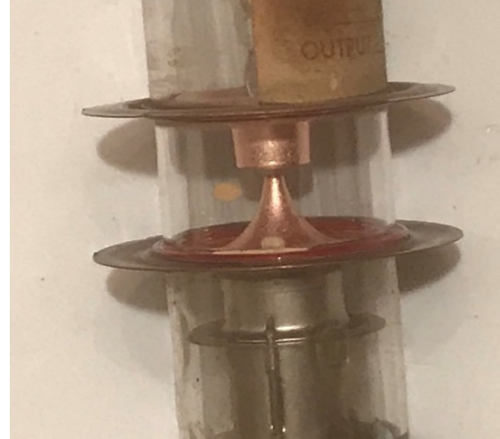
Fig 12. The annular diaphragms forming the drift space (rhumbatron) in which the electron stream is bunched
