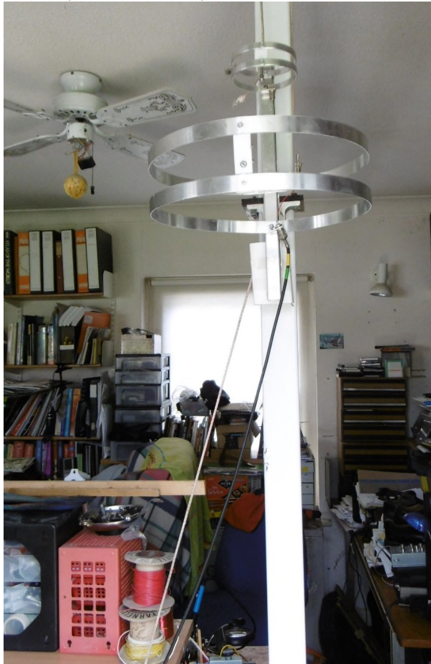
Figure 2. Low profile 145 and 432 MHz slot antennas in the shack, rope up/down able.
