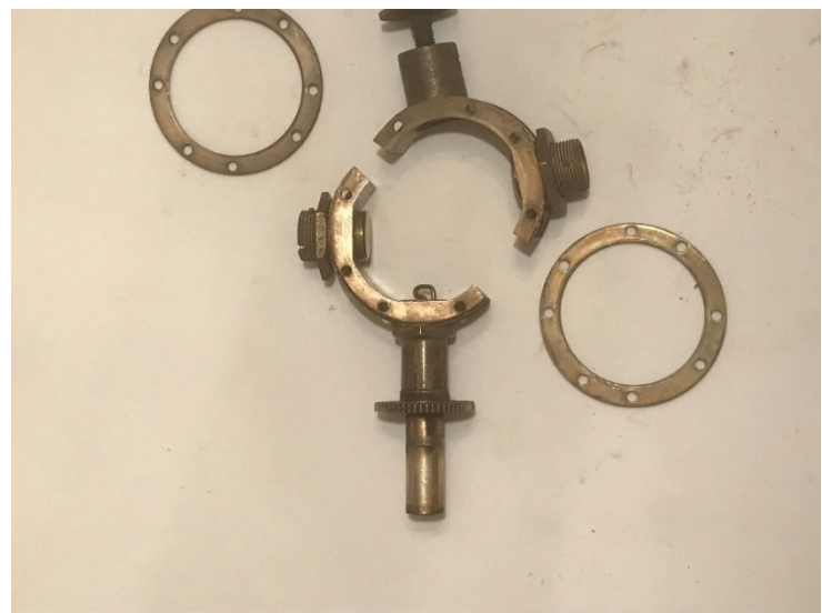
Fig 8 The substantial cast aluminium mounting frame, which also served to heat sink the klystron
