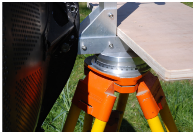
The Turntable and main dish mount. The scale in degrees is a stick-on metric measuring scale, 1 degree equals 1mm - the diameter over the scale is 4.511"
