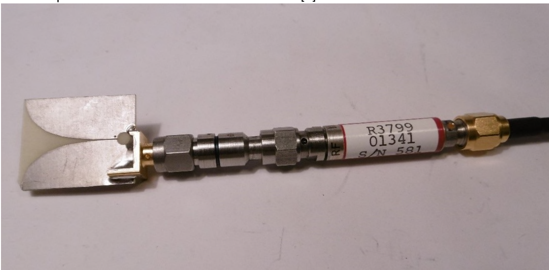
Figure (5a) Back detector and ~10 – 30 GHz Vivaldi. Note I have used an inline attenuator in this instance. Back diodes can be expensive. This one is obsolete I discovered [3] but not blown.
