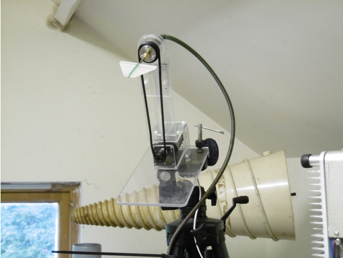
Figure (5a) Back detector and ~10 – 30 GHz Vivaldi. Note I have used an inline attenuator in this instance. Back diodes can be expensive. This one is obsolete I discovered [3] but not blown.
