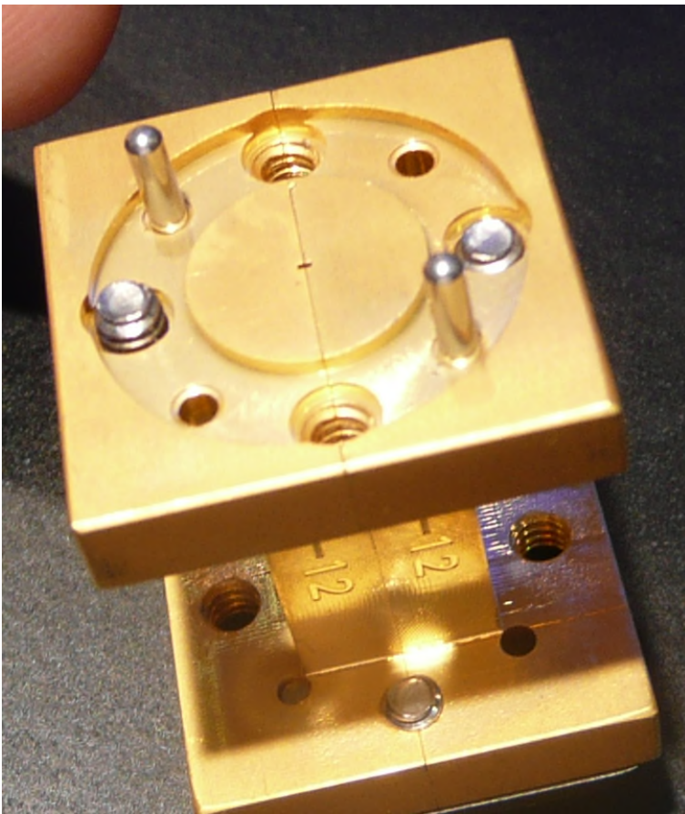
Figure (6c) We can also do the same thing using TE 10 mode waveguide at 300GHz. Here the need to electroform the surface to reduce loss is essential
