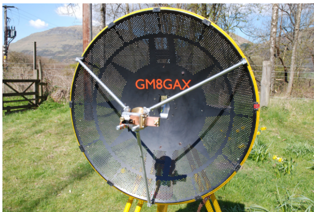
The dish, these were rejects from a MoD supplier, you can see the lug that is out of position on the rim of the dish still with the original red marker tape.
