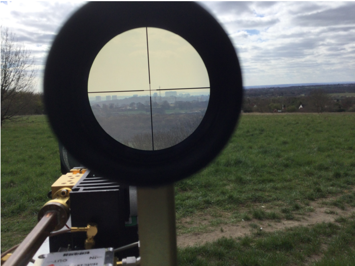
View through the TX scope toward Minster from Danbury. The mast is on the former Marconi/BAE radar site. The tower blocks further on at Southend. In practice azimuth had to be adjusted further to the left (East).
