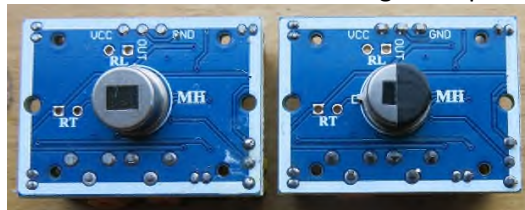
Figure 3(a) Front side of HC-SR501 PIR board with "insect eye" lens removed from sensor
