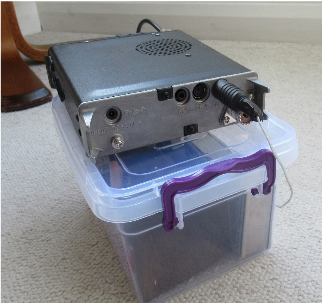
Photo 3: Rear view, PTT link and antenna horn
