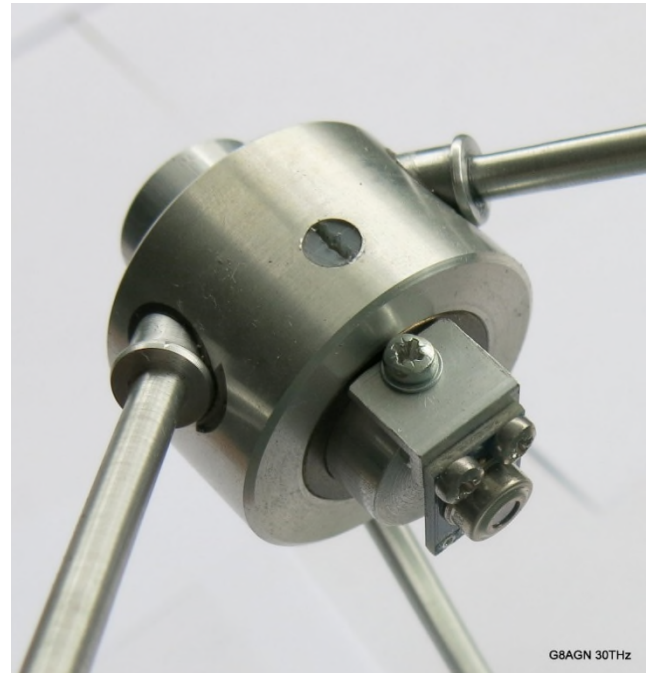
Figure 5 Melexis sensor mounted at the focus of the parabolic reflector
