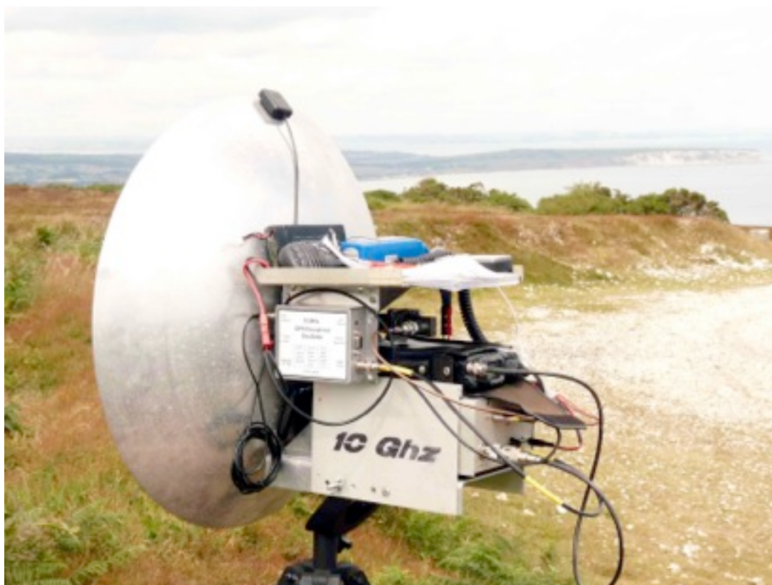
G0PEB/P entering the UK Microwave Society 10GHz contest 29th June 2014. FT-817 & DB6NT Mk3 transverter, including GPSDO. Antenna : 60cm dish with Penny feed. Power O/P :- 200mW. Best DX : G3XDY @229km Location: St Boniface Down, Isle of Wight IO90JO.
