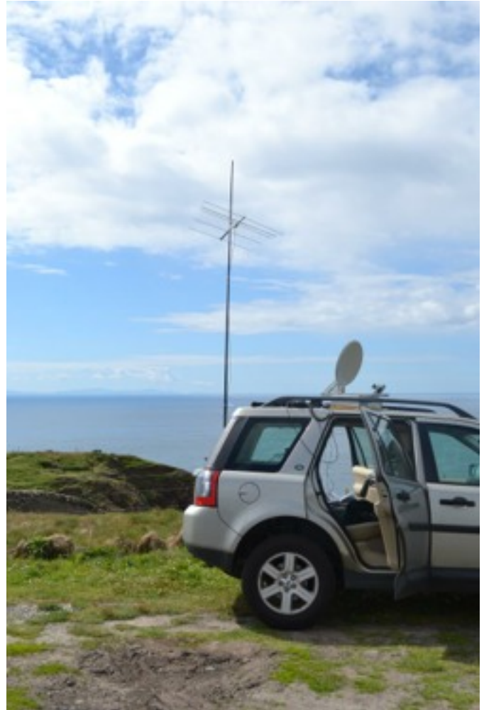
Photo – Isle of Man in background (2m talkback antenna pointing at it) but the dish is looking at the GB3NGI beacon!
