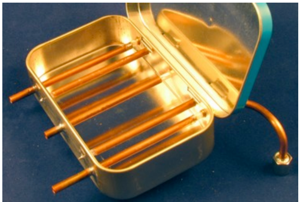
Figure 9 - Interdigital filter with coupled-rod input and semi-rigid cable end connections
