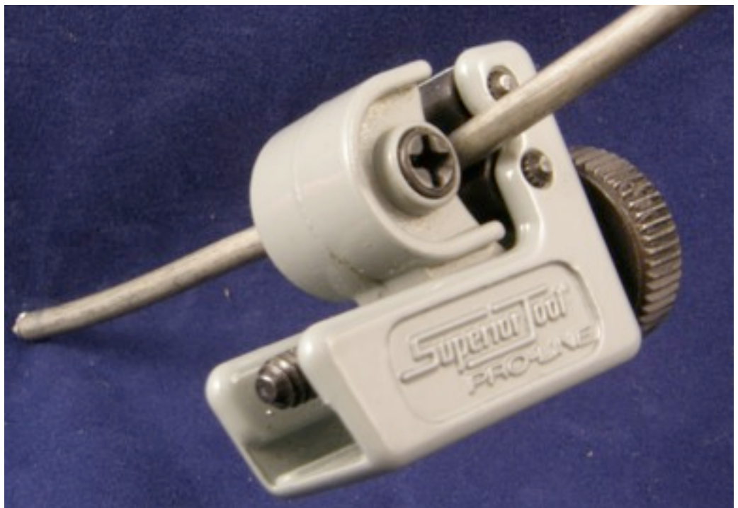
Figure 11 – Preparing semi-rigid coax with miniature tubing cutter
