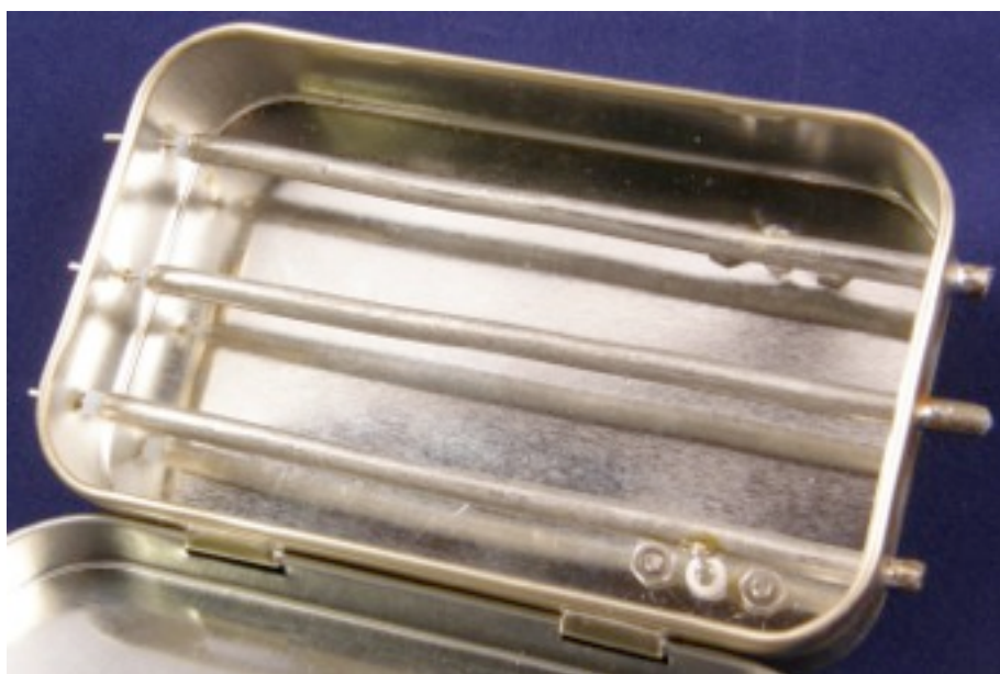
Figure 1 – 432 MHz Combline filter in Altoids tin
