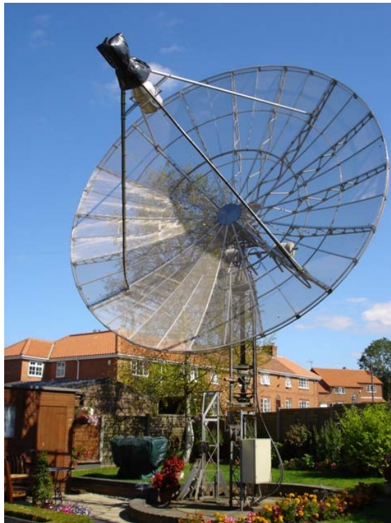
G4CCH Wire mesh steerable dish for 2.3GHz Global EME (Moonbounce Operation), Lincolnshire
