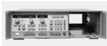
axis. Not a big problem as you can convert it with an op-amp on dual rail supplies. You can also use an op-amp if you need a greater voltage swing. You can use an op-amp to work the other way around as the popular 141 spectrum analyser sweep output has a +/- 5V swing – yes you can use the first LO as a limited range sweeper.
