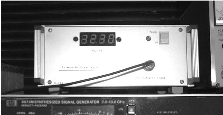
A common technique used to determine voltages at Radio Frequencies is to employ a diode detector circuit designed specifically for the frequencies and power levels of particular interest. The resulting dc voltage is proportional to the RF voltage, however this relationship is not linear due to diodes having a "Square Law Characteristic". Custom scales can be made for Analogue Panel meters but some form of linear conversion is necessary for a digital display.
