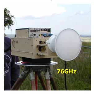
operational system makes an interesting challenge. Antenna systems can reduce in size as the frequency increases but the narrow beam antennas require good pointing accuracy. In higher frequencies there are challenges associated with frequency accuracy, stability, transmitter output power and receiver sensitivity. But these challenges drive the interest and there is a good community of willing helpers to assist.
