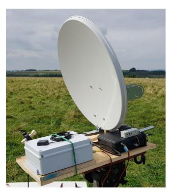
Around 2.5W maximum drive is needed at 144 MHz for 2W output at 24GHz.
