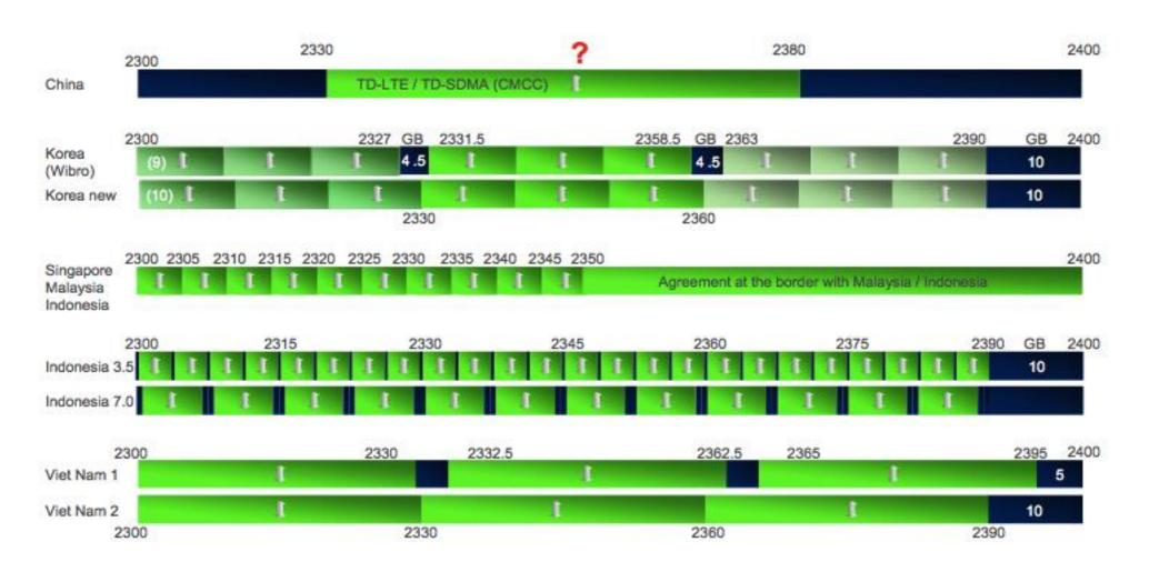
Each country has opted for different standards and channel widths; in some cases guard bands have been set up...
