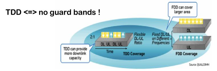
In the case of FDD operation, there are two carrier frequencies, one for UL transmission and one for DL transmission. During each frame, there are consequently 10 UL subframes and 10 DL subframes, and UL and DL transmission can occur simultaneously within a cell.
