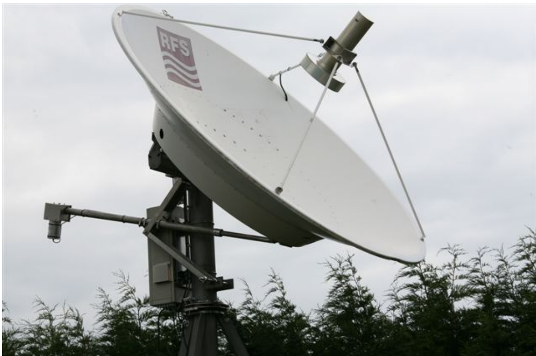
Figure 1: The complete ON0EME beacon installed on top of a 10 ft shipping container
