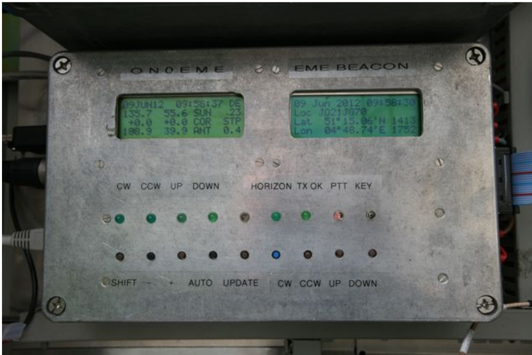
Figure 7: Beacon controller including antenna positioner, GPS receiver and beacon keyer
