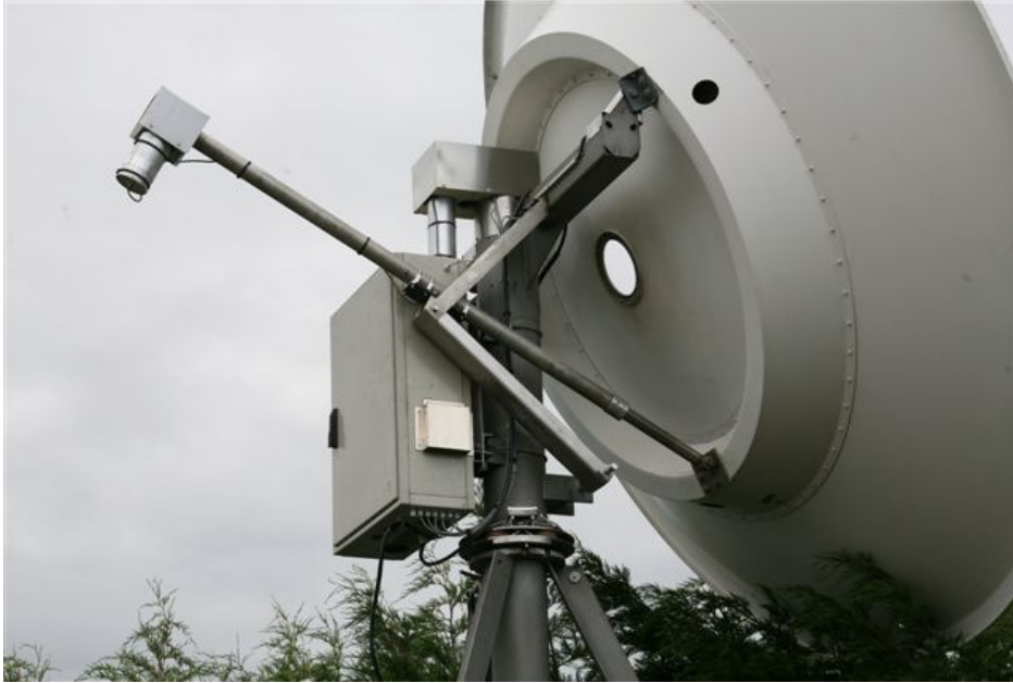
Figure 3: Back structure of the antenna with AZ and EL motors and equipment box
