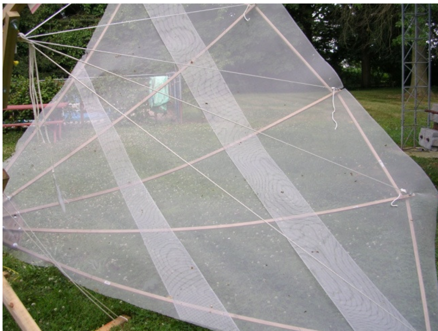
Figure 8: Aluminum screening is tied to spokes using wire
