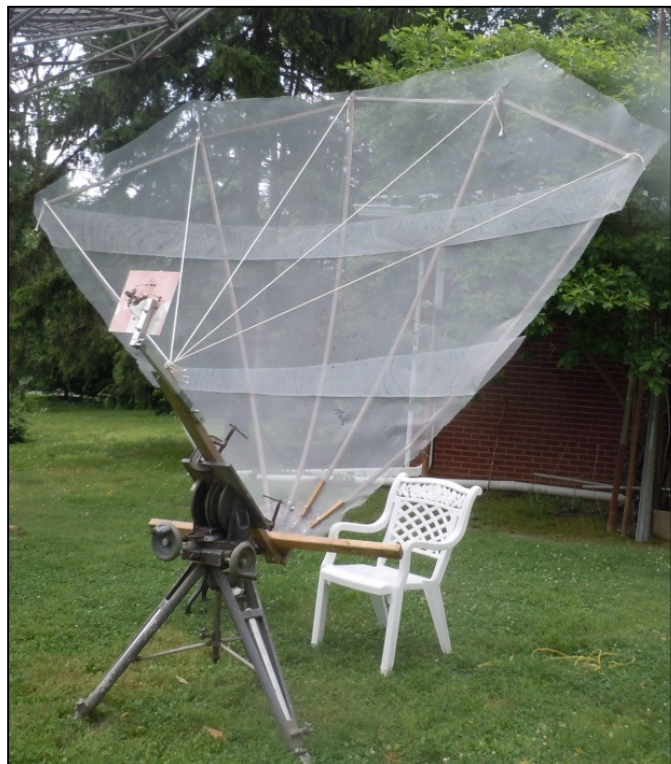
Figure 1: 7.5 ft offset stress dish
