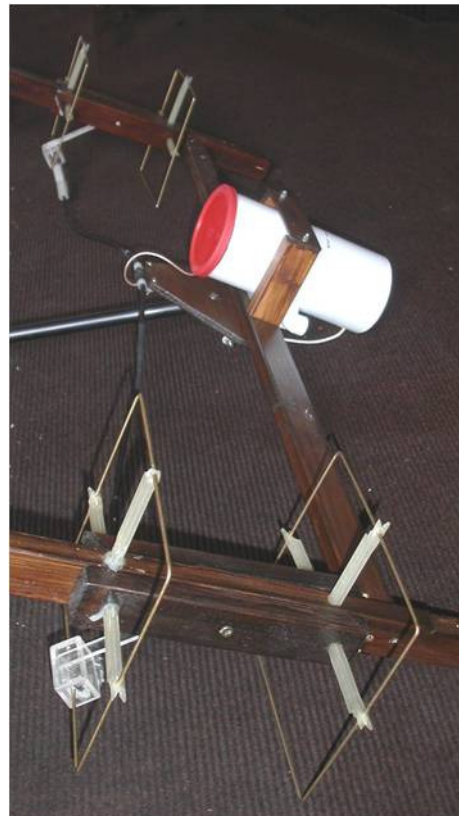
Figure 5: Stacked Quagis and head amplifier
