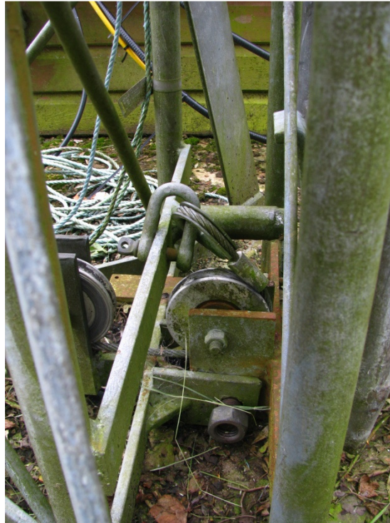
Figure 6: Mechanical advantage system on the author's tower – left hand pulley is for cable guidance, but the right-hand pulley provides a mechanical advantage of 2
