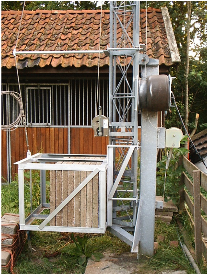
Figure 2: Tilt-over tower and ground post at PE1BTX, showing the counterweight cage and one of the two lifting balloons (see text)
