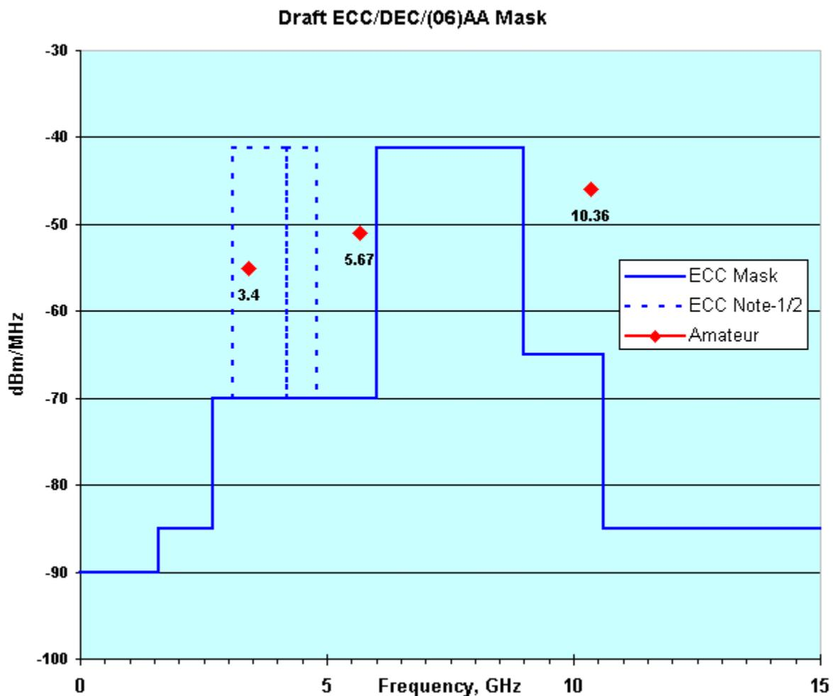
The plot above is mask level specified in the Annex of the Draft Decision, compared to the protection levels that Report 64 determined are necessary for the Amateur Services
