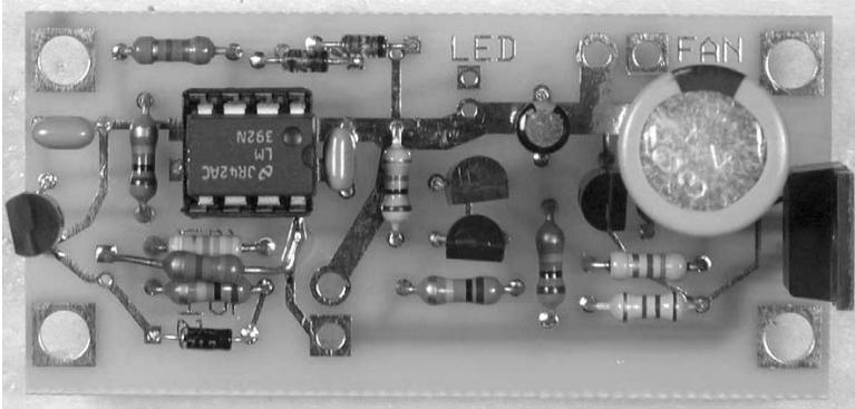
Glue, or use a dab of heat sink compound and clamp it on. A heat sink takes some time to heat and cool, so the fan will not change speed instantaneously, but will speed up as the heat sink heats. More important, it will continue running at higher speed until it brings the heat sink temperature down, gracefully slowing down as things cool. U2 need not be mounted on the printed circuit board, but may be mounted remotely, on the heat sink; twist the wires together, and
