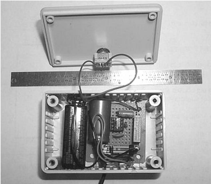
The "Dasher" was designed and built within two week of our recent 24 gigahertz Marathon. It was built purely out of a need for self-preservation. Standing on a cold windy hilltop and sending (not so well formed) dashes for 5 to 10 minutes at a time with a straight key was, to say the least, uncomfortable. I refrained from using my home station keyer because of the added weight and bulk to an already pretty hefty "portable" station. I wanted something small, light and self contained.
