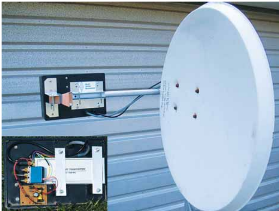
Figure 1: Quickstarter mounted on the feed arm of a surplus TVRO Offset dish with internal shot inset
