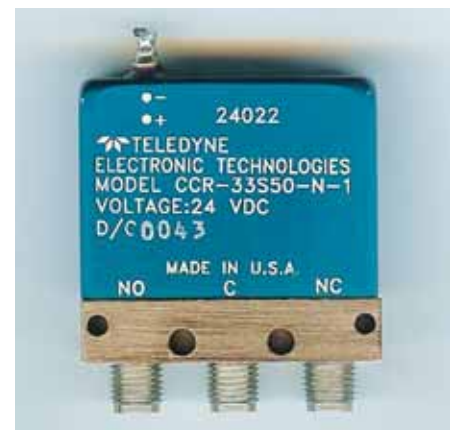
Figure 2: A typical SMA relay suitable for use at 10GHz
