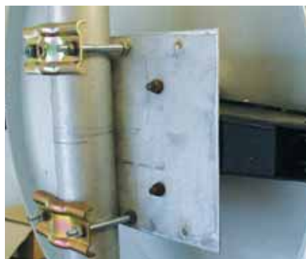
Figure 9: Mounting arrangement for a surplus TVRO dish using a plate.
